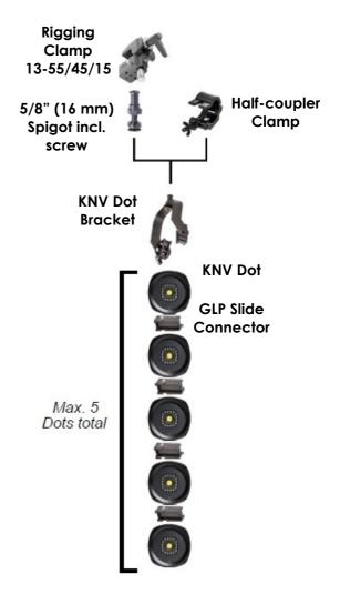
Figure 13. Single column of 5 x KNV Dots suspended using a KNV Dot Bracket
