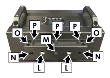
Figure 6. PSU mounting points
