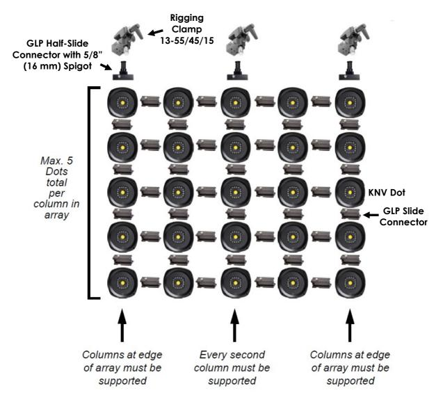
Figure 16. KNV Dots array, every second column independently supported
