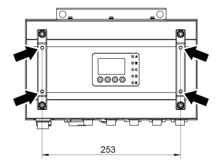
Figure 31. Using PSU handles for mounting
