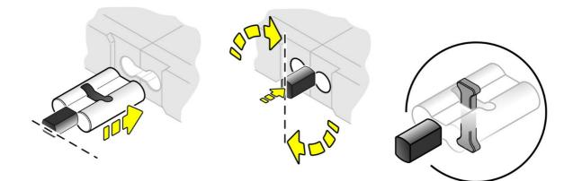
Figure 20. Locking mechanism on KNV Line mechanical connectors
