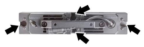
Figure 18. Mechanical connector channels on KNV Line
