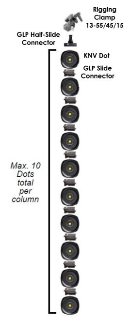
Figure 14. Single column of 10 x KNV Dots suspended using a GLP Half-Slide Connector
